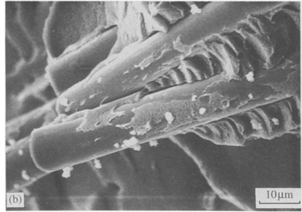
Figure 6 As Fig. 5 after immersion in 85 °C water for 100 h. (Broken at room temperature.)
